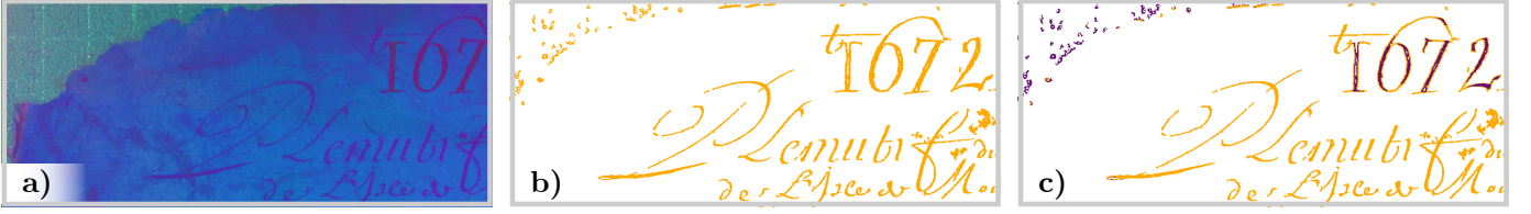
Fig. 1: A detail from the MS-TEX MSI 1 database (z97). A pseudo color image a), the binarization result b) and the foreground estimation c). While yellow pixels indicate definitive foreground, violet pixels are marked as uncertain and thus not used for the ACE signature estimation.
