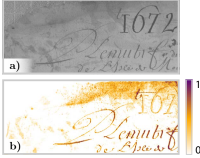
Fig. 3: The F2 channel (500nm) from the MS-TEX MSI 1 database a) and the resulting target detection image b)
