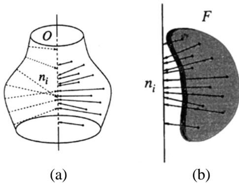
**Fig. 5:** Surface normals  $n_i$  of a rotationally symmetric object  $O$  intersect the axis of rotation  $a$ ; this should be true for complete objects (a) and for its fragments (b) (from[Hal97]).
