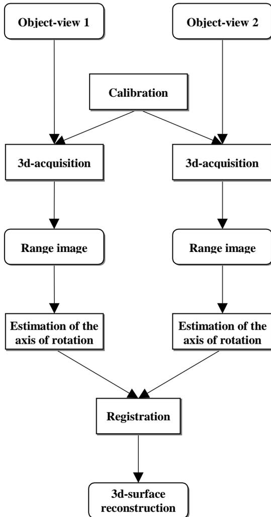
**Fig. 1:** Overview on 3d-reconstruction from two object views
