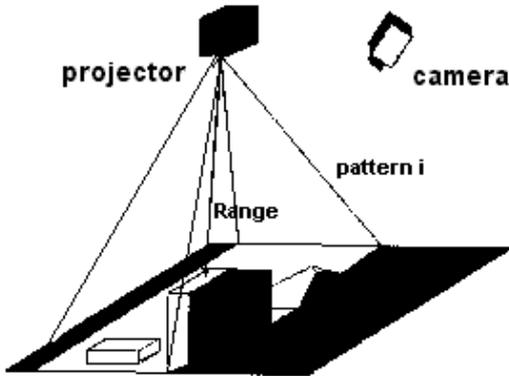
**Fig. 2:** Configuration with light projector, camera and object
