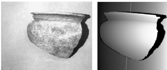
**Fig. 6:** Intensity image (left) and range image (right) of a fragment with rotational axis of the front-view
