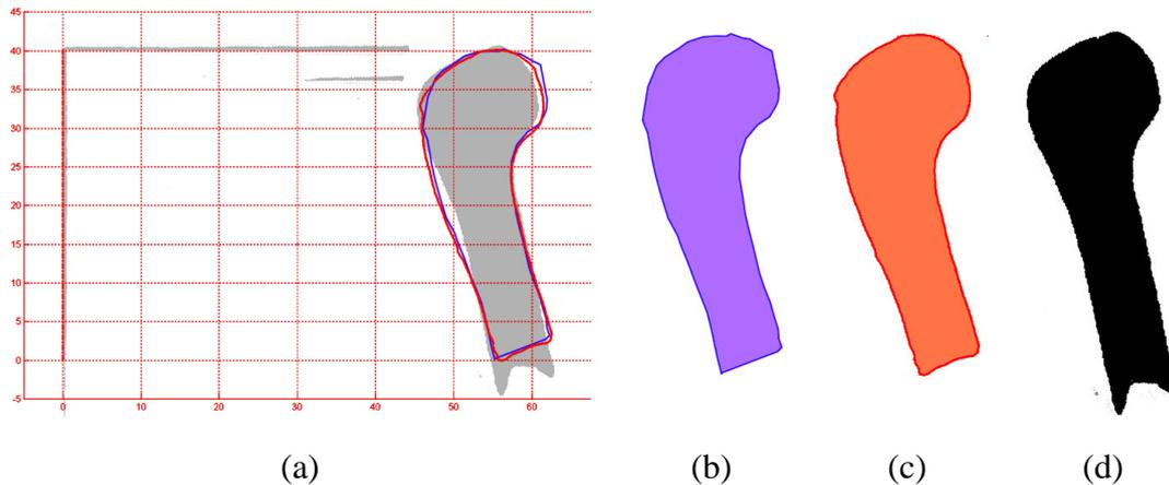
Figure 6: (a) Profile Lines extracted at the same point of the sherd in respect to the rotational axis (equals  $y$ -axis), acquired by the *profilograph* (b), the 3D-Scanner (c) and the manual drawing (d).
